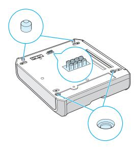
4 Place the printer over the tray, aligning the feet on the printer with the positioners in the optional tray.
